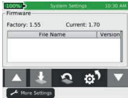
You can have more than one version of firmware on the SD-Card – all firmware files on the SD-Card will be displayed on this screen. Use the Up ▲ and Down ▼ buttons to scroll through multiple firmware files.
